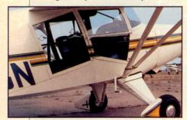
There is no mistaking the heritage of the fabriccovered steel fuselage.
